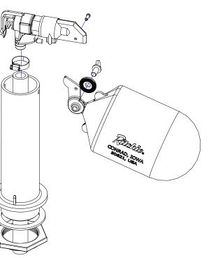
J. **Final Water Connection**– Connect the top of the supplied hose to the valve, cut hose to proper length, and slip onto the barb fitting of the valve assembly. Clamps and fittings are furnished to secure the connection.
