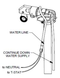
3/4" Valve Cable Heater Setup
