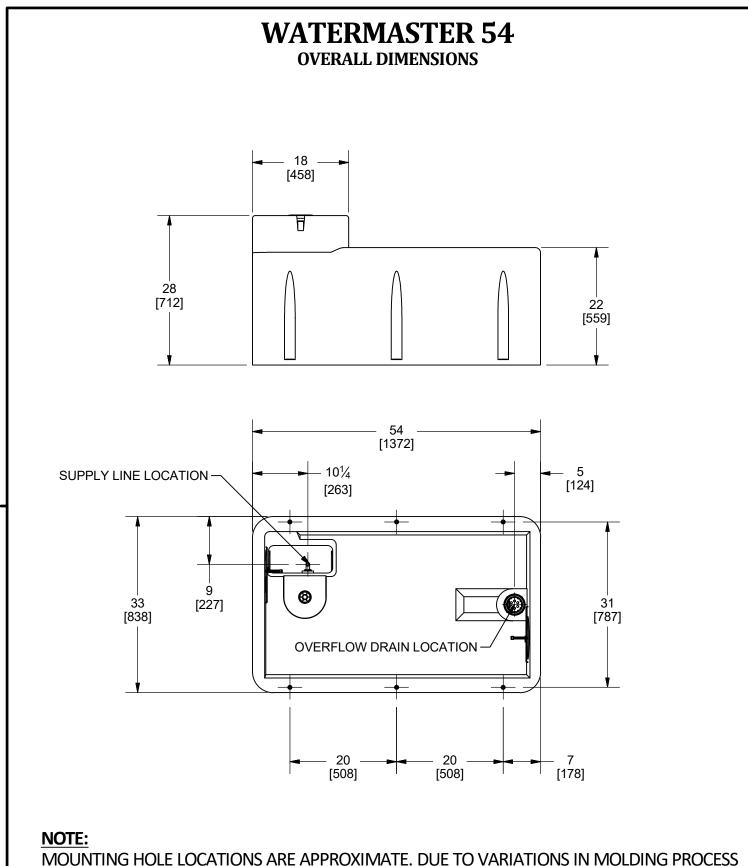
MOUNTING HOLE LOCATIONS ARE APPROXIMATE. DUE TO VARIATIONS IN MOLDING PROCESS IT IS NOT RECOMMENDED TO USE THIS DRAWING FOR LOCATING CONCRETE ANCHORS. IT IS RECOMMENDED TO WAIT UNTIL UNIT IS AVAILABLE FOR MEASUREMENT.
