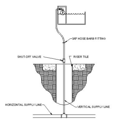
the fountain to allow for servicing. If your facility is cold in the winter, a using a Ritchie Thermal Tube as your riser will provide optimum protection to the vertical supply line against frost and freezing.
