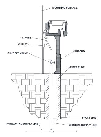
D. **Water Supply Through Wall** - Through wall supply lines should be sized to account for pressure drop, relating to distance, and located to prevent tampering by livestock. A one-inch supply pipe is recommended. A shut-off valve should be located at the fountain to allow for servicing. If your facility is cold in the winter, additional cold climate protection will be required.
