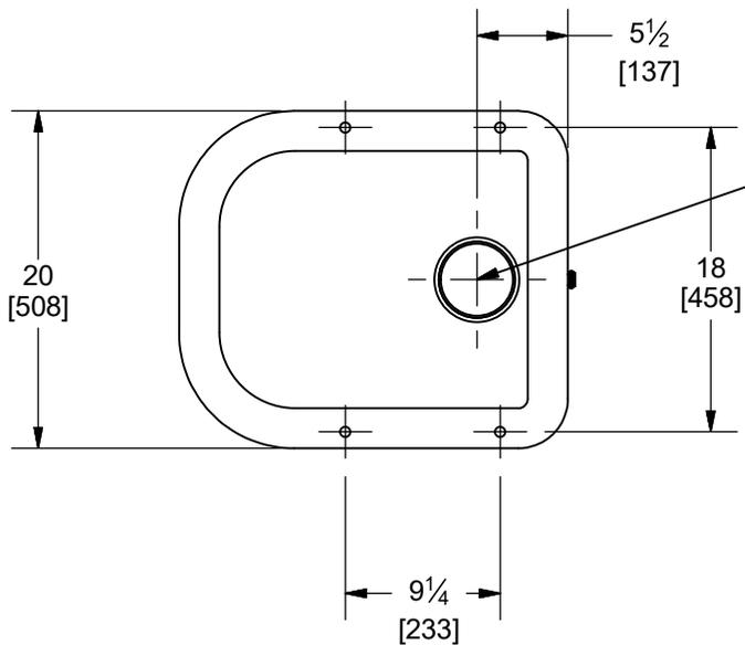
CONNECTION MAY BE MADE THROUGH THIS ACCESS IF SUPPLY LINE IS RAN UNDER GROUND
