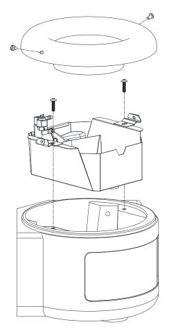
After the Stall Fount is securely mounted to the wall and all supply connections are made you can reinstall the trough with the Phillips
