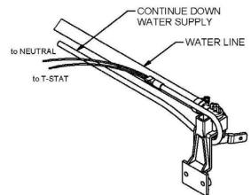
**K. Electrical Connection** - The electrical installation should be made and maintained by a qualified electrician conforming to national and local codes. A means for disconnection must be incorporated in the fixed wiring in accordance with the wiring rules. For wiring connections, see wiring diagram. Make connections according to the wiring diagram below.
