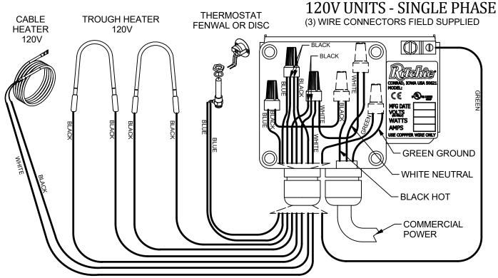
WARNING - CHECK NAMEPLATE FOR CORRECT VOLTAGE. ONLY CONNECT 120VAC TO 120V UNITS. WIRING DIAGRAM SHOWN WITH 2 HEATERS - QUANTITY MAY VARY
