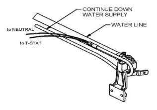
**H. Electrical Connection** –A means for disconnection must be incorporated in the fixed wiring in accordance with the wiring rules. For wiring connections, see wiring diagram. Make connections according to the wiring diagram below.
