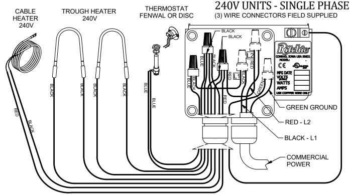
WARNING - CHECK NAMEPLATE FOR CORRECT VOLTAGE. ONLY CONNECT 230-240VAC TO 240V UNITS. WIRING DIAGRAM SHOWN WITH 2 HEATERS - QUANTITY MAY VARY
